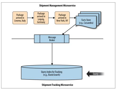
*Figure 5-4. Data flow in command-query responsibility segregation (CQRS)-based model for Shipping, Inc.*
