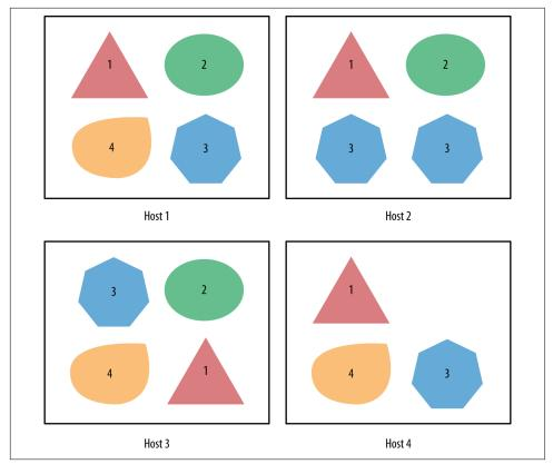
Figure 6-1. Microservice deployment topology with nonuniform service distribution
